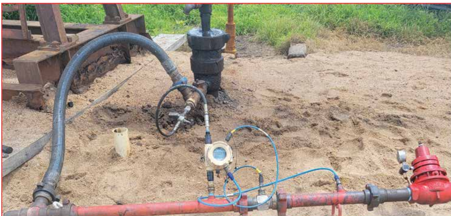
With this setup we can measure and record gas you have on the annulus.
